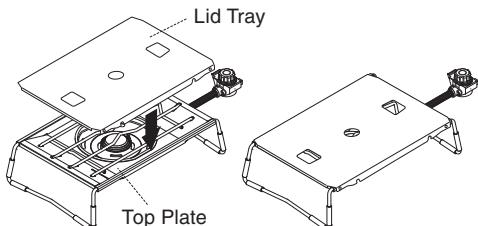
For details on how to attach the top plate, refer to the Flat Burner Instruction Manual.
